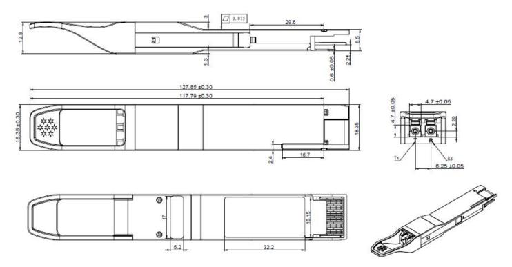
Figure6. Mechanical Specifications
