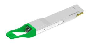
KP-FEC. These modules are designed to operate over single mode fiber systems using LAN-WDM 8 wavelengths. The electrical interface uses a 76 contact edge type connector. The optical interface uses duplex LC connector. The Common Management Interface Specification (CMIS) for QSFP DD modules, This module incorporates Fibertop Technologies proven circuit and EML technology to provide reliable long life, high performance, and consistent service.
