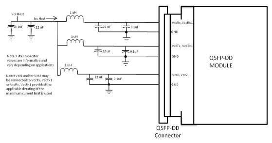
Figure3. Host Board Power Supply Filtering
